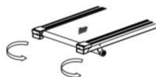
Enabling the belt - screw counterclockwise
